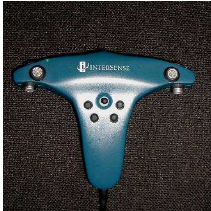
Figure 2.4: Photograph of the InterSense™ IS-900 six degree of freedom wand. This was used as the interaction device for the immersive treatments of this study.
