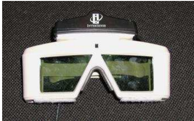
Figure 2.3: Photograph of the CrystalEyes™ LCD shuttered glasses with an InterSense™ InterTrack motion tracker mounted on top. This pair of glasses was worn by participants during the immersive treatments. A similar pair glasses without the motion tracker was worn by test participants during the desktop treatment.
