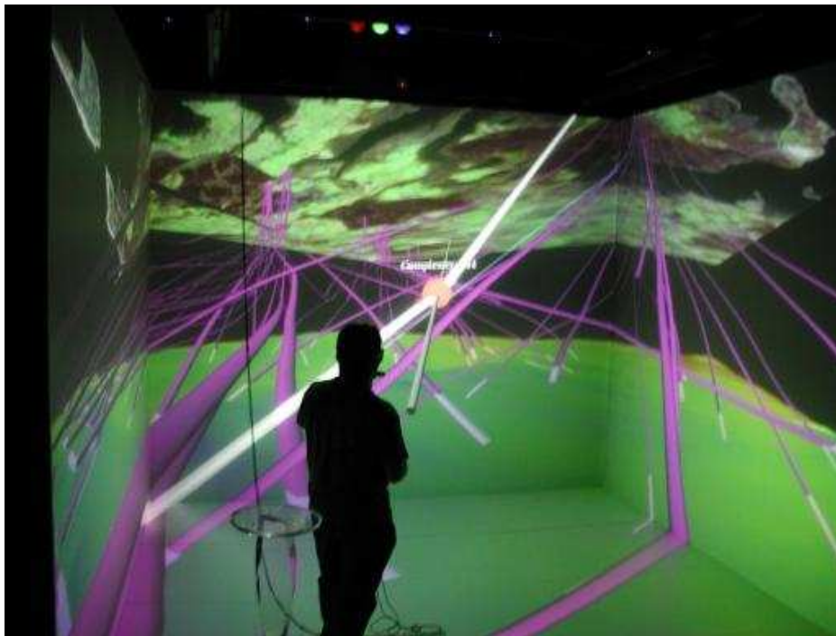
Figure 3.12: Photograph of a IDP user interacting with the virtual world using the ray-casting technique. A virtual ray extends from the wand and virtual objects can be moved and rotated by when intersected by the ray.
