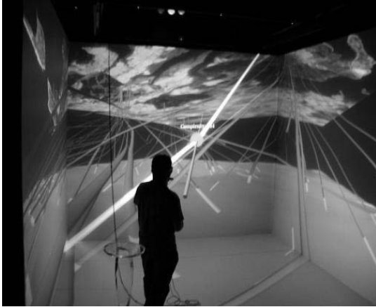
Figure 2. Photograph of a IDP user interacting with the virtual oilfield inside the IVE using the ray-casting technique.
